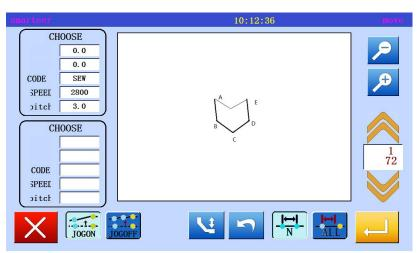
\* With the mobile key to determine the starting point (B point) and the end point (E point).
