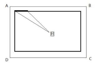
In a polygon mode, input offset sewing (with overlapping reinforcement), set the offset distance: 5.0mm, direction: right, overlapping seam end reinforcement mode: 1, the number of times: 3)
