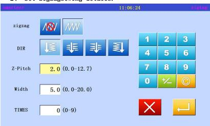
Input with overlapping suture reinforcement end lambdoid suture, the circle. The offset width of the figure is 5.0mm, the transfer amount is 3.0mm, the direction is left, and the implementation of an overlapping reinforcement, to carry out the three stitch overlapping sewing. (black overlaps the reinforce part)
