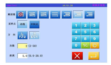
\* Select and input multiple layers of sewing, direction, distance, and number of times
